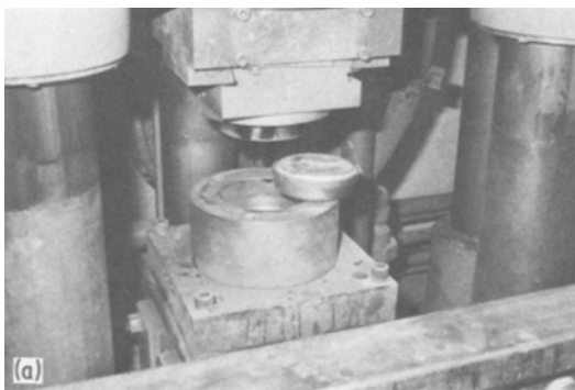
Figure 6 Photographs of the forging die in the hydraulic press and the parts produced. (a) shows a disc-shaped part about 115 mm in diameter and about 40 mm in height. (b) Shows the steel ring insert used in the lower die-half to produce the reduced cross-section disc-shape on the right.
